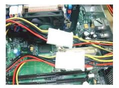
The connected cables for two PL-P3/SMPs.
